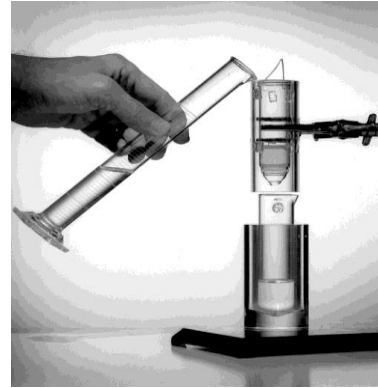
Original Tc-99m generator 1958 shown without shielding
